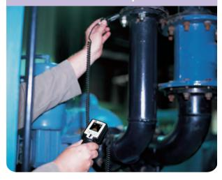
Leak detection with focus tube
